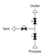
The F68 and F69 are integrally forged, onepiece valve assemblies for primary isolation of pressure take-offs, where the valve is mounted directly to the vessel or process pipe. Instruments may be directly mounted to the valve outlet or alternatively remotely mounted with gauge lines/ impulse pipe work.
