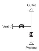
The HD27 and HD27MK are integrally forged one-piece block and bleed assemblies for primary isolation of pressure take-offs, where the valve is directly mounted to the vessel or process pipe. Instruments may be directly mounted to the valve outlet or alternatively remotely mounted with gauge lines/impulse pipe work.
