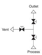
The F29 and F33K are integrally forged, one-piece double block and bleed assemblies for primary isolation of pressure take-offs where the valve is mounted directly to the vessel or process pipe. Instruments may be directly mounted to the valve outlet or alternatively remotely mounted with gauge lines/impulse pipe work.
