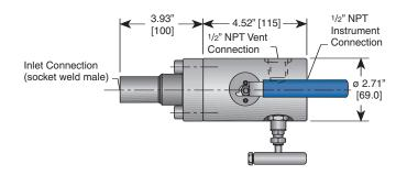
The P62 is an integrally forged one-piece block and bleed assembly for primary isolation of pressure take-offs, where the valve is either screwed or welded directly into the vessel or process pipe without the need for a flanged connection. Instruments may be directly mounted to the valve outlet or alternatively remotely mounted with gauge lines/impulse pipe work.
