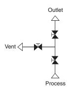
The HD33 and HD33MK are integrally forged one-piece double block and bleed assemblies for primary isolation of pressure take-offs, where the valve is directly mounted to the vessel or process pipe. Instruments may be directly mounted to the valve outlet or alternatively remotely mounted with gauge lines/impulse pipe work.
