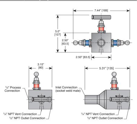
The HD29 is an integrally forged one-piece double block and bleed assembly for primary isolation of pressure take-offs where the valve is either screwed or welded directly into the vessel or process pipe without the need for a flanged connection. Instruments may be directly mounted to the valve outlet or alternatively remotely mounted with gauge lines/impulse pipe work.
