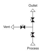
The F66 and F73/F73K are integrally forged, one-piece valve assemblies for primary isolation of pressure take-offs, where the valve is mounted directly to the vessel or process pipe. Instruments may be directly mounted to the valve outlet or alternatively remotely mounted with gauge lines/impulse pipe work.
